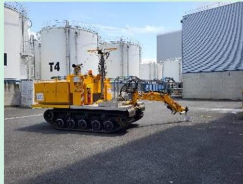
X-ray probe placement by the remotely operated robot ERASE
