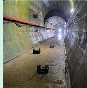
Visual inspections and radiological mapping in long tunnels using a chain of relay robots
